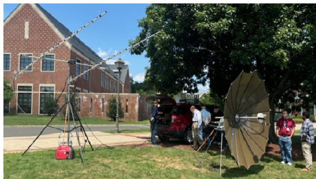
KA6U EME Rover with 70 cm Xpol Yagis and 2.4 m dish
